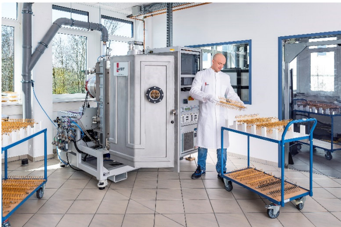
Image 3: PVD plasma reactor for nano-structured surface modifications with Au, Pd, Pt, Ag, Cu, etc.
