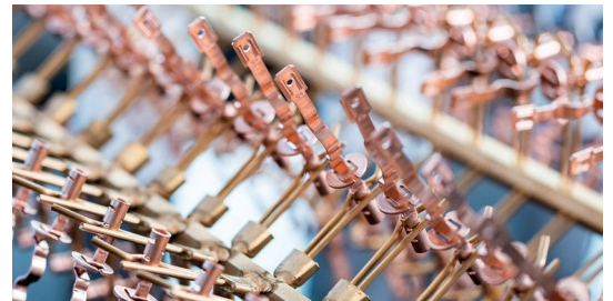
Stamping and bending technology for optimum signal conductors made of copper (Cu), silver (Ag) or aluminium (Al)
