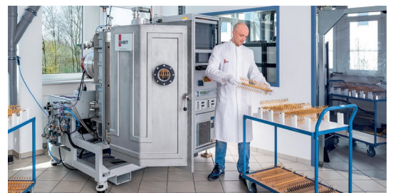
PVD plasma reactor for nano-structured surface modifications with Au, Pd, Pt, Ag, Cu, etc.
